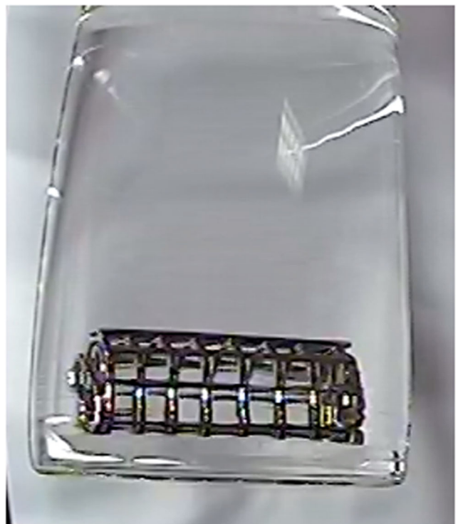
Fig. 13. For the round bottom vessels, a portion of the view of the JP sinker is obscured when the camera is mounted at an angle approximately 90 degrees to the central axis of the vessel
