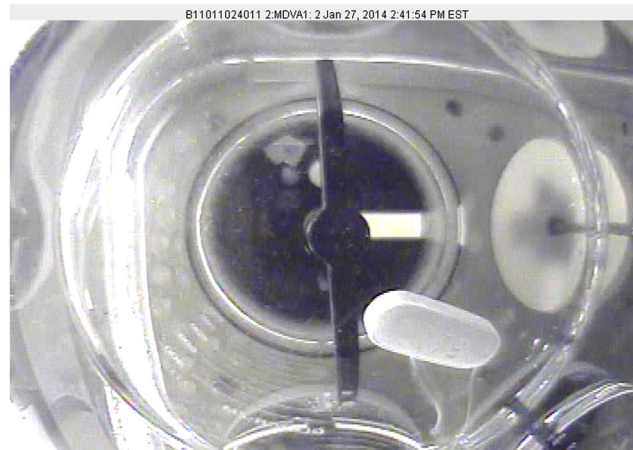
Fig. 3. Using such a system, one can easily identify the presence or absence of the dosage forms in the vessel
